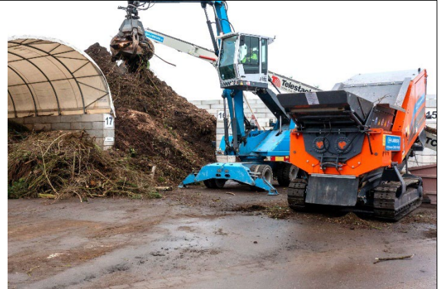
The EKOMAXX 800 mobile twin-shaft shredder in daily use for shredding green waste
