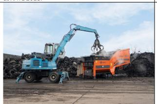
The mobile version of the ARJES TITAN 900 has already proven itself in use with the Fuchs MHL 320. At RATL 2023, ARJES will present its stationary solution for this system combination.
