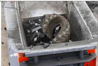
The power of the asynchronously running paddle shafts shreds even the heaviest scrap tires
