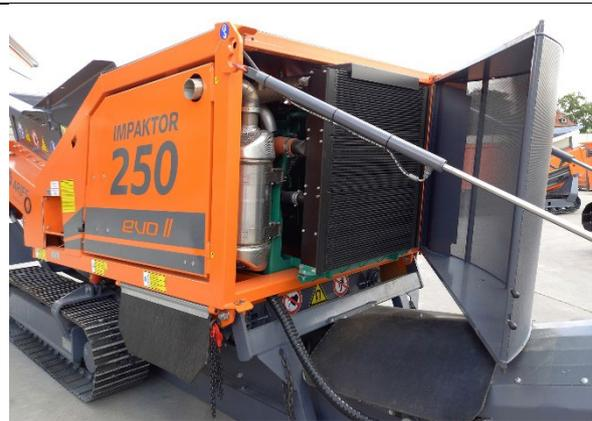
High air suction volume and optimal accessibility of the engine for service, maintenance and cleaning thanks to the new semi-circular radiator grille
