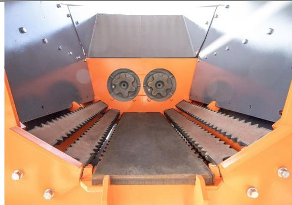
By inserting or removing the plates, the gap width may be modified and thus the final grain size adjusted. In case of worn cutting blades, the plate can be rotated and reinserted several times.
