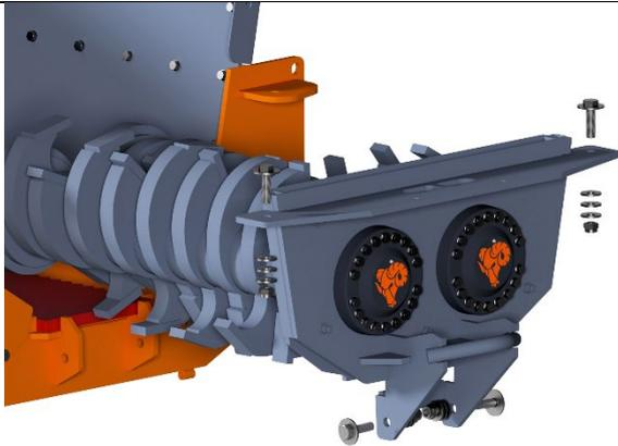
The improved quick-change cassette ensures a significantly longer operating time as the pressure during the crushing process is no longer exerted on the fastening bolts, but on the entire machine.
