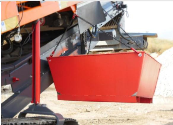
Height adjustable permanent magnet for effective FE separation including discharge container
