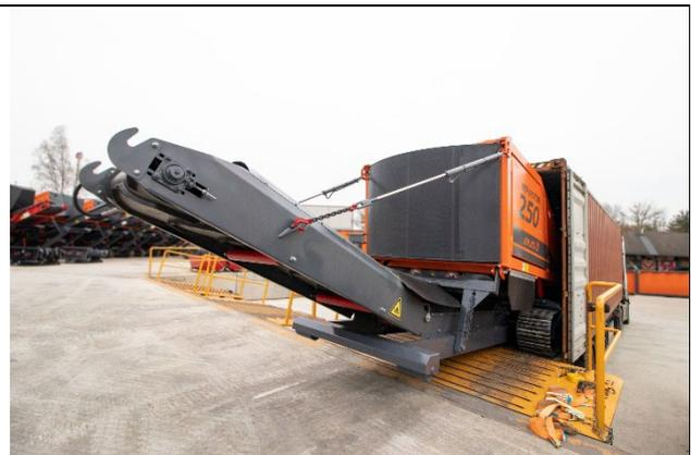
Due to the reduced transport height to approx. 255 cm, sea container collections are possible without dismantling the hopper walls and the maximum loading height for trucks is generally not exceeded.
