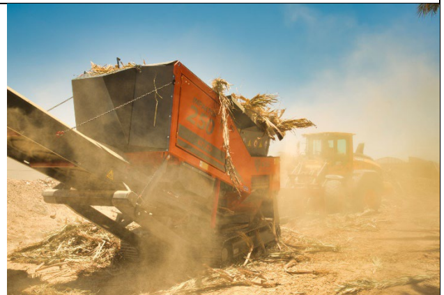
Temperatures above 45°C as well as fine dust and sand place heavy stress on the machine
