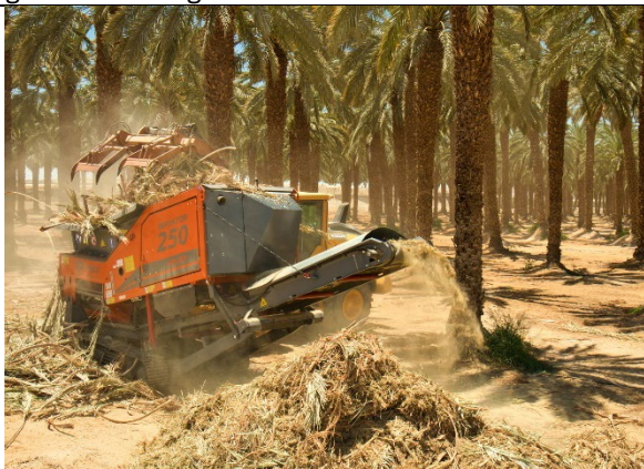
Making full use of the ARJES IMPAKTOR 250 evo for shredding palm fronds
