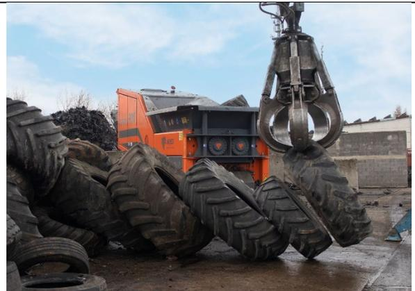
Even heavy EM tyres with a high proportion of steel mesh are shredded with the TITAN 900
