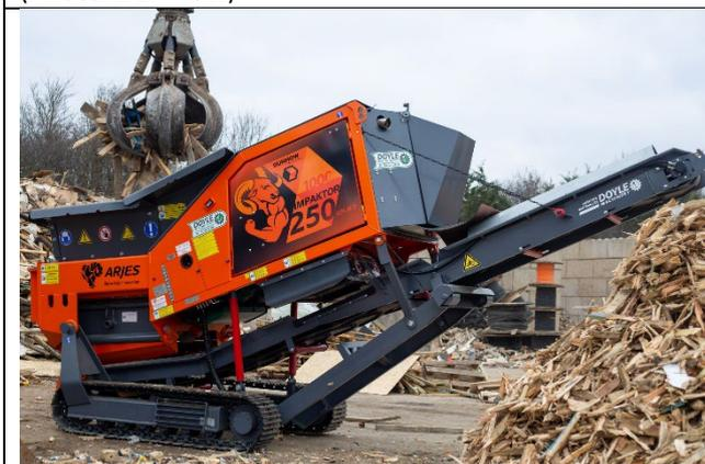
IMPAKTOR 250 evo during the first test run - shredding waste wood (Photo: Dunmow)
