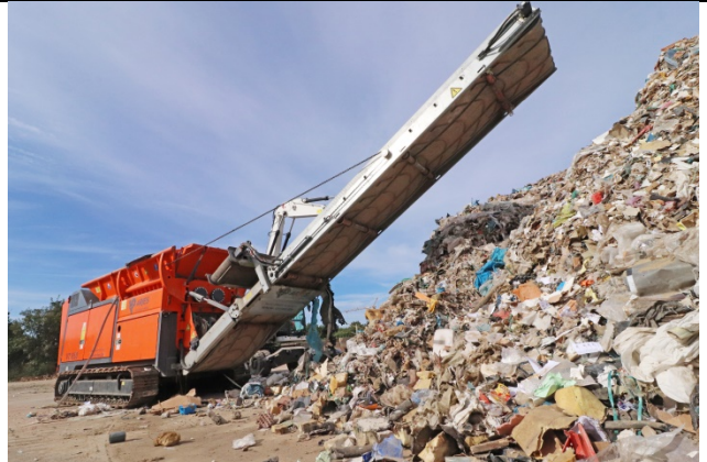
Extended discharge belt ensures a high discharge cone of the shredded material
