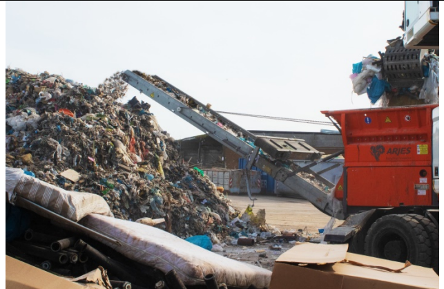
Various mixed materials, including mattresses, are shredded by the VZ 850 DK without any problems
